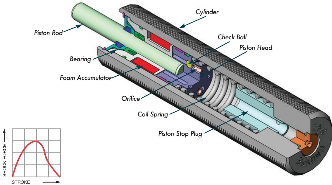
**Constant orifice area damping** (dashpot) provides the largest shock force at the beginning of the stroke when impact velocity is highest. These shock absorbers provide high-energy absorption in a small, economical design.
